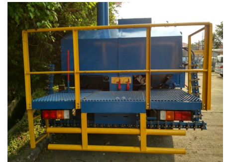
Operator Platform for easy inspection during spraying
