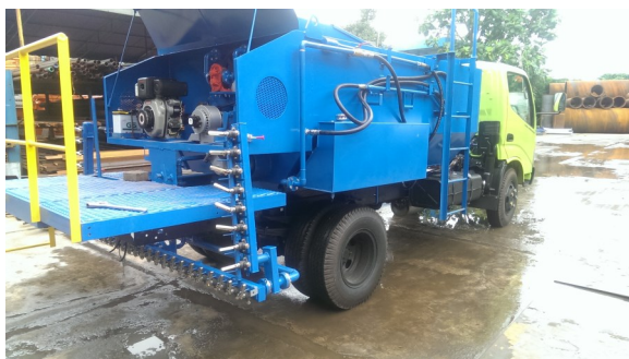
Spray Bar can be folded from total 4000 mm to 2400 mm wide
