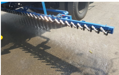
Multi Nozzles, individually can be turned off
