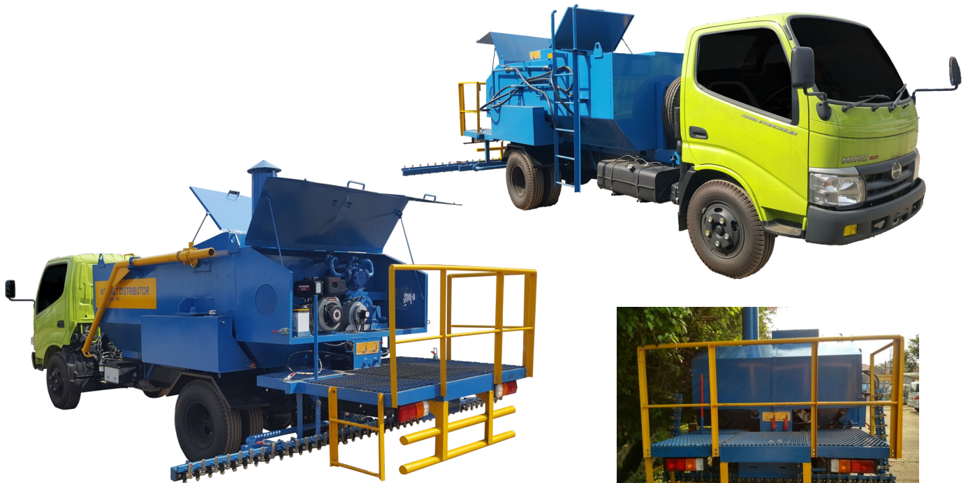
Operator Platform for easy inspection during spraying
